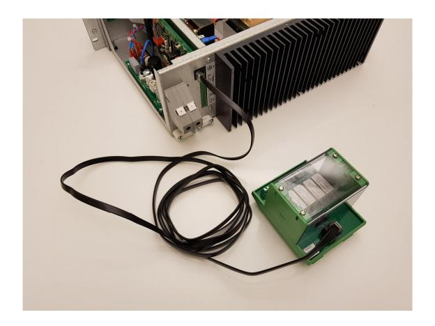
Connect the enclosed cable between pin 16 and chassis/earth if earth fault monitoring is to be enabled.
