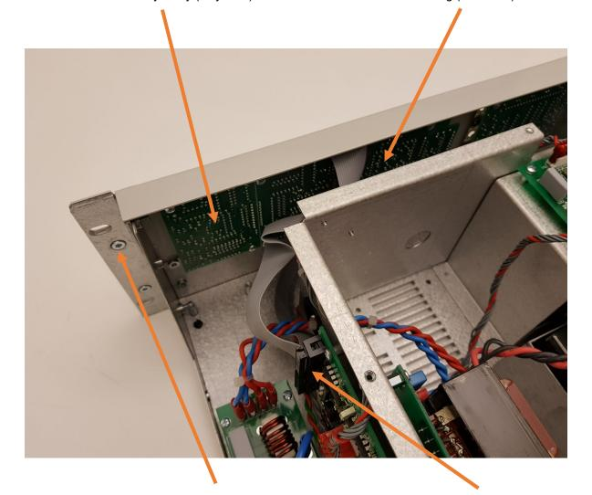
Unscrew these screws on each side of the rectifier (4 pcs in total) to remove front panel.
