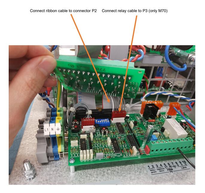
Replace the screws with spacers and attach relay board onto the spacers (only M70).
