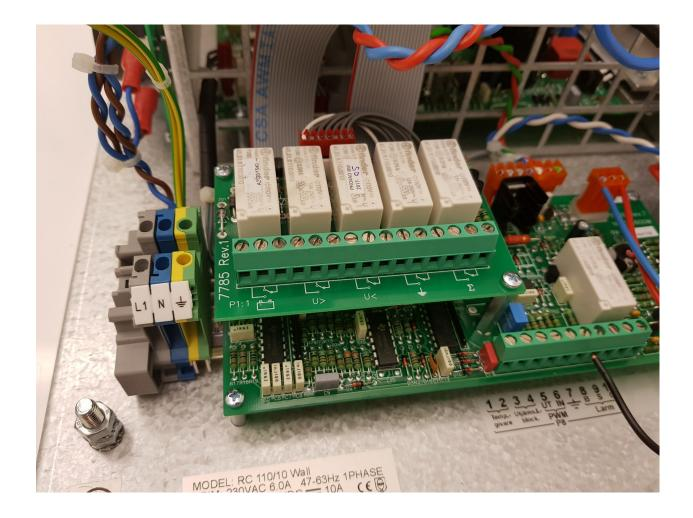
Connect the enclosed cable between pin 7 and chassis/earth if earth fault monitoring is to be enabled.
