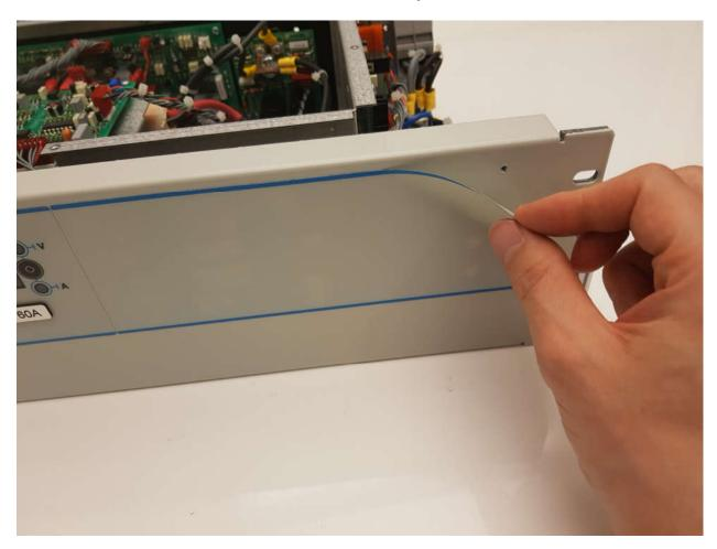
Remove the cover and front panel of the rectifier and mount the board for monitoring and the board for relay delay (only M70).
