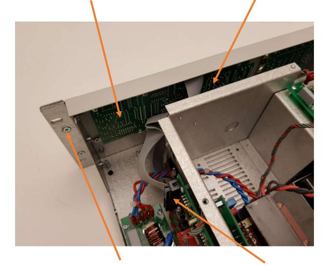
Unscrew these screws (4 pcs) in order to remove front panel P2
